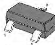
Marking Code: A7 SOT-23 Plastic Package
